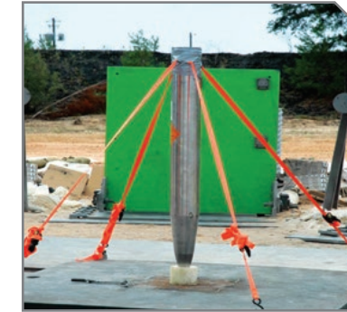
Test For Casing Fragments Damage On Wall Panels
